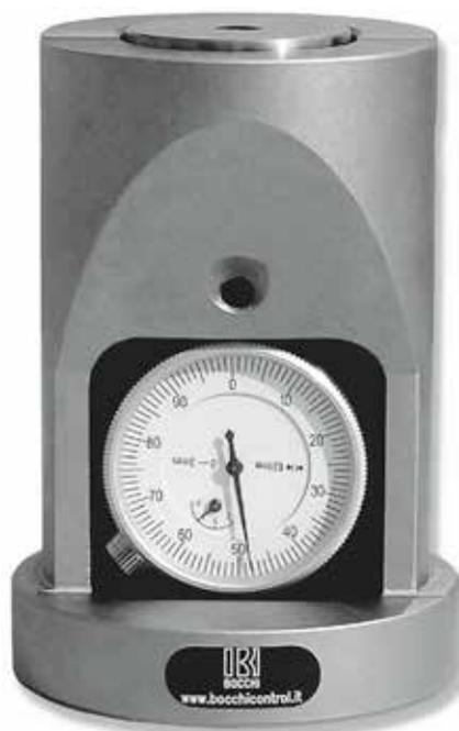
**Setting tool instrument** with one fixed and one mobile part. Acting on the mobile part with the tool, the dial indicator gives the measurement variation. Suitable for use on machine tools to check the exact length of the tool compared to the working surface. Supplied in case with dial indicator.
