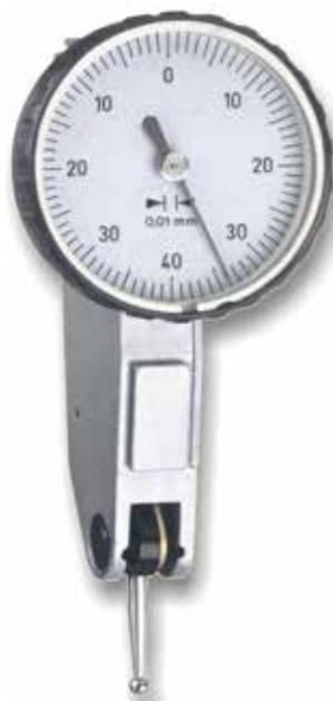
**Test indicator.** Ruby-mounted gear movements give maximum precision but the test indicator is also shockproof. Automatic inversion of the direction of measurement without a switch to anticlockwise direction of the indicator. Supplied with three guides for attachment to comparator holders for greater versatility. Complete with  $\varnothing$  2 mm ball probe tip and  $\varnothing$  8 mm connector. Manufactured as per DIN 2270 form A. Supplied in case. .
