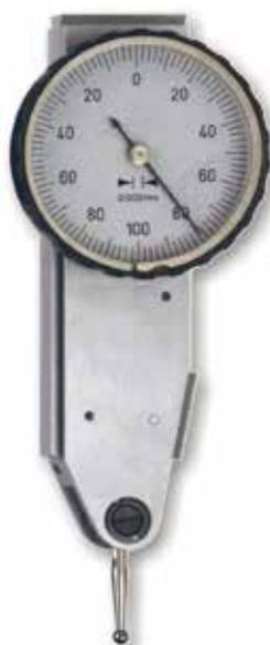
**Test indicator.** Ruby-mounted gear movements give maximum precision but the test indicator is also shockproof. Automatic inversion of the direction of measurement without a switch to anticlockwise direction of the indicator. Supplied with three guides for attachment to comparator holders for greater versatility. Complete with  $\varnothing$  2 mm ball probe tip and  $\varnothing$  8 mm connector. Manufactured as per DIN 2270 form B. Supplied in case.
