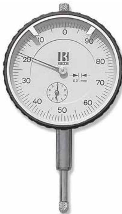
*Shockproof dial indicator with anticlockwise dial. Advanced technology transmission mechanisms. Shocks received by the probe are not transmitted to the internal mechanisms so that precision remains constant. Rotating bezel with tolerance markers. Manufactured as per DIN 878. Supplied in case.*
