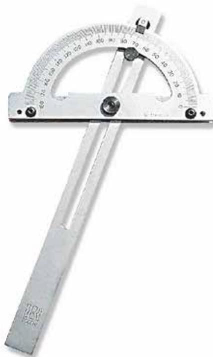
*Adjustable goniometer. Made from galvanically treated, anti-corrosion steel. Angle capacity 10-170° with 1° graduations. Etched, easy to read, long-lasting. With double base.*
