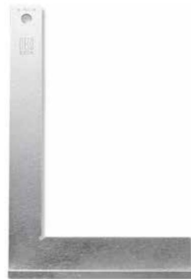
*Square with stock in non-deformable steel. The reduced section makes it easier to handle and is suitable for blacksmiths and carpenters. Entirely ground on the faces and protected by anticorrosion treatment. High precision. Made with tolerances  $\pm(0,04 + L/5000)$  mm.*
