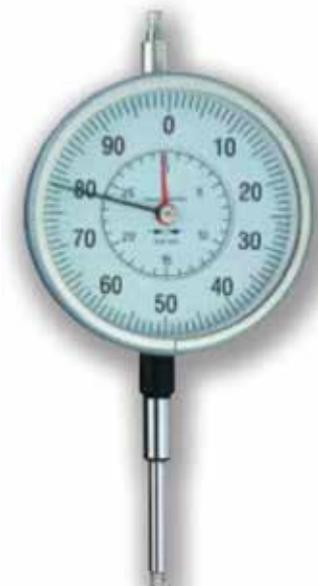
*Shockproof dial indicator with big dial. Robust metal housing and construction, assure the accuracy on all range. Insulated internal mechanisms to avoid shocks. The bezel together with the outer dial can be rotated to set zero in any position. Manufactured as per DIN 878.*
