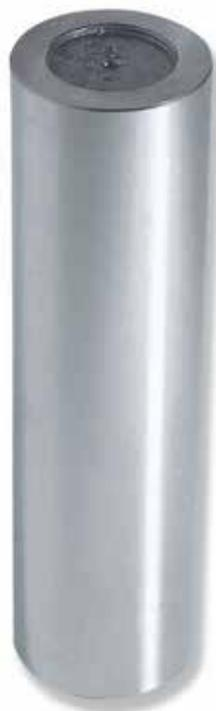
*Steel gauging cylinder for testing 90° squares and mechanical parts. Entirely ground. Placed in front of a light, any error in the item being checked will let light pass through the gap. Manufactured as per DIN 875/0. Hard chrom plated upon requirement.*
