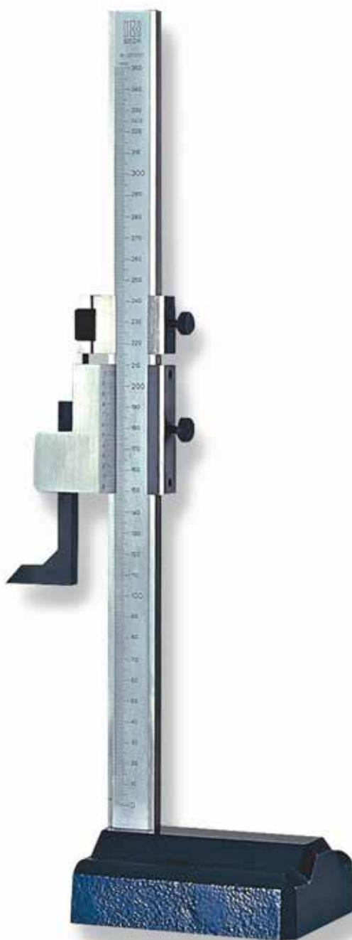
**Height gauge** in hardened stainless steel. Graduated, satin-chromed scale with etched, precision graduation. Easy to read, long-lasting. Raised slide for easy movement. One-piece slider with micrometric adjustment. Slider locking screw. Squared scribing point with carbide tip. Heavy, painted cast iron base for stability with anti-slip grooves. Serial number. Manufactured as per DIN 862.
