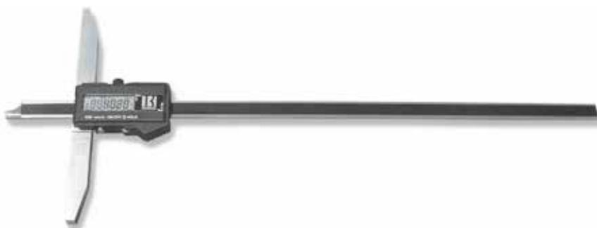
**Digital readout depth measuring caliper** in hardened stainless steel. State-of-the-art electronics. mm/inch conversion. Set to zero in any position. RS232C output to printer port. Slider locking screw. Serial number. Manufactured as per DIN 862. Supplied in case.
