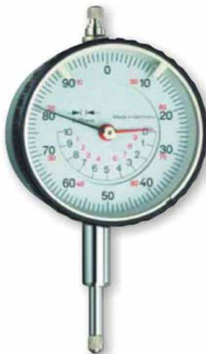
*Both pointers are concentrically arranged on the dial gauge shockproof dial indicator. This allows particularly clear reading. Manufactured as per DIN 878.*
