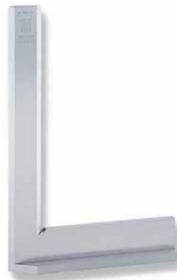
*Knife edge square with stock in hardened stainless steel. The two chamfered and lapped sides allow more accurate visual control. Entirely ground. High precision, made and tested to very strict procedures. Serial number. Manufactured as per DIN 875/00. Supplied in case.*
