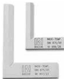
*High precision square with bevelled internal edge. Made from hardened stainless steel. Manufactured as per DIN 875/00. Supplied in sheath.*
