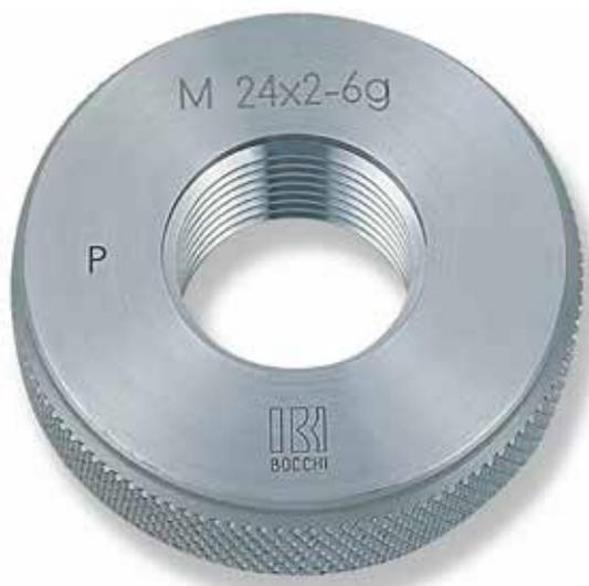
*Thread ring gauges. In high wear-resistant steel-chrome alloy. Core-hardened, tempered and stabilised. Normally constructed gauges for the following thread types: Metric, Withworth, Cylindrical gas, Tape gas, Acme, American unified UNC, UNF, UNEF. The ring gauge to tolerance 6g in the standard versions.*
