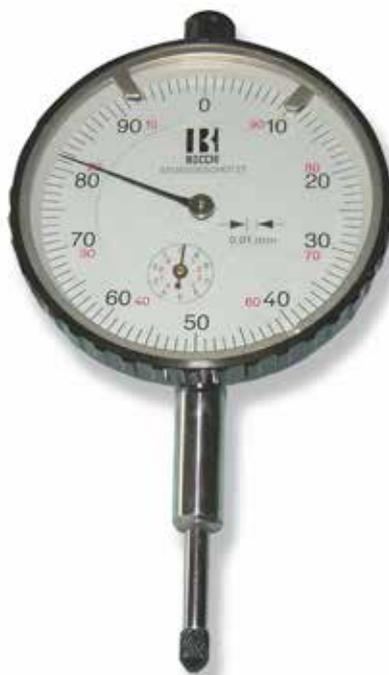
*Shockproof dial indicator with advanced technology transmission mechanism. Shocks received by the probe are not transmitted to the internal mechanisms so that precision remains constant. Rotating bezel with tolerance markers. Manufactured as per DIN 878. Supplied in case. Rubin contact.*
