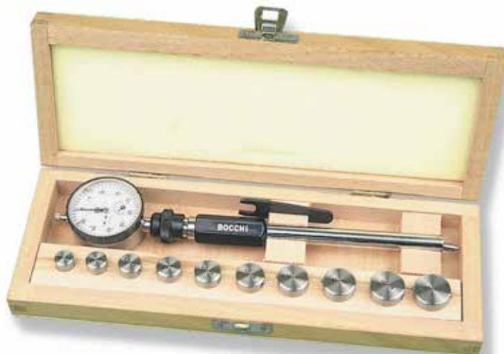
**Bore gauges with hardened steel contact surfaces for small bores.** The travel on the contact surfaces is transmitted via a needle in hardened steel a 1:1 ration.
