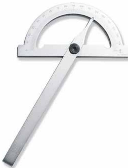
*Fixed pin goniometer. Made from galvanically treated, anti-corrosion steel. Angle capacity 0 – 180° with 1° graduations. Etched, easy to read, long-lasting.*
