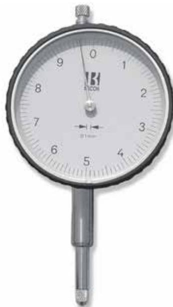
**Shockproof, decimal dial indicator** with advanced technology transmission mechanism. Shocks received by the probe are not transmitted to the internal mechanisms so that precision remains constant. Rotating bezel with tolerance markers. Manufactured as per DIN 878. Supplied in case.
