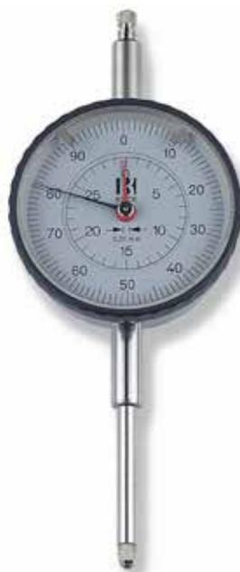
**Shockproof, long range dial indicator.** Sturdy construction ensures constant precision across the whole measurement range. Internal mechanisms are insulated separately to protect against shocks received by the probe. Rotating bezel with tolerance markers. Manufactured as per DIN 878. Supplied in case.
