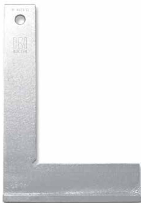
**Square with stock** in non-deformable steel. The **base is made from a monoblock piece** not assembled making this a very strong square suitable for heavy carpentry work. Galvanic treatment protects it from oxidation.
