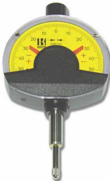
*High precision dial indicator with measurement to 0,001 mm with protective cap. Entirely shockproof. Moving parts are mounted on ball-bearings for sensitivity and a minimal response time. The upper button allows adjustment of the indicator in any position. Tolerance markers and lifting cable. Manufactured as per DIN 879. Supplied in case.*
