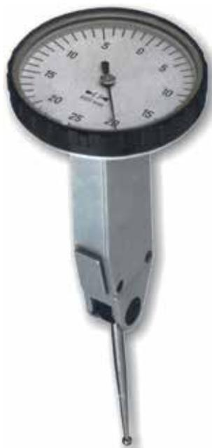
**Test indicator.** Ruby-mounted gear movements give maximum precision but the test indicator is also shockproof. Automatic inversion of the direction of measurement without a switch to anticlockwise direction of the indicator. Supplied with three guides for attachment to comparator holders for greater versatility. Complete with Ø 2 mm ball probe tip and Ø 8 mm connector. Manufactured as per DIN 2270 form C. Supplied in case. .
