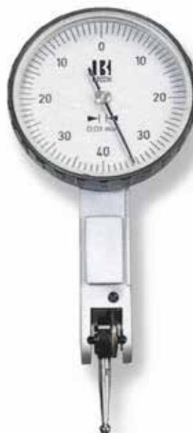
**Workshop test indicator.** Ruby-mounted gear movements give maximum precision but the test indicator is also shockproof. Automatic inversion of the direction of measurement without a switch to anticlockwise direction of the indicator. Supplied with three guides for attachment to comparator holders for greater versatility. Complete with Ø 2 ball probe tip and Ø 8 connector. Length of probe 12 mm. Manufactured as per DIN 2270 form A. Supplied in case.
