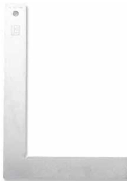
*Flat square in non-deformable steel. The reduced section makes it easier to handle and is suitable for blacksmiths and carpenters. Entirely ground on the faces and protected by anticorrosion treatment. High precision. Made with tolerances  $\pm(0,04 + L/5000)$  mm.*
