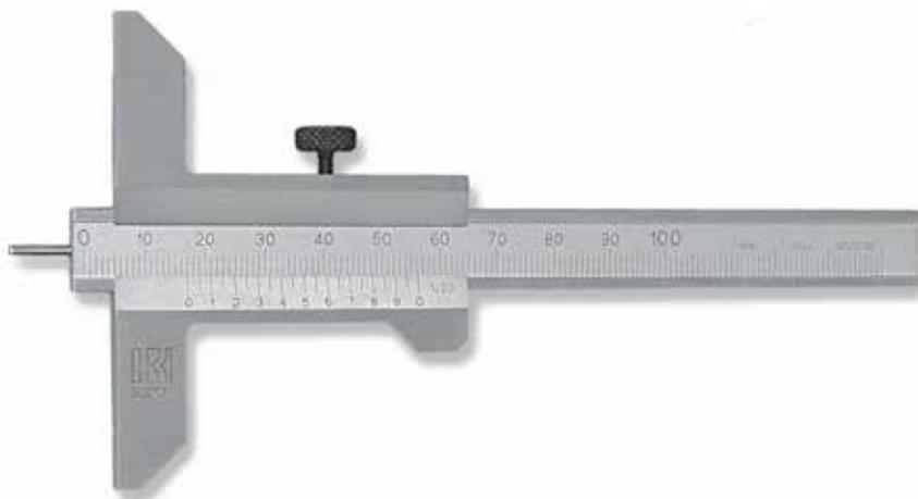
*Depth measuring monoblock caliper in hardened stainless steel. Satin-chromed readout scale. Etched, precision graduation, easy to read and long-lasting. Raised slider for easy movement. Slider locking screw. Serial number. Manufactured as per DIN 862. Supplied in case. Point  $\varnothing 2 \times 10$ .*
