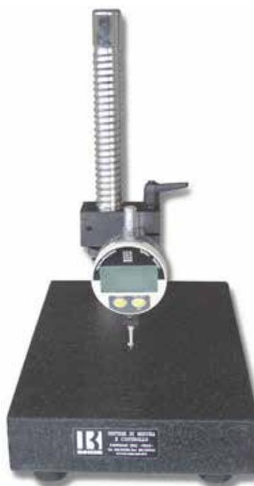
*Dial indicator stand with granite rectangular base. Dial indicator holder unit on horizontal rod with fine adjustment. The vertical column in chromed steel is threaded for micrometric adjustment and is equipped with an horizontal arm able to reach all points of the base. Precision of the base  $\pm 2,2 \mu\text{m}$ . Supplied without dial indicator.*
