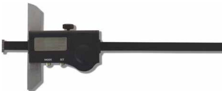
*Digital readout depth measuring caliper in hardened stainless steel. State-of-the-art electronics. mm/inc conversion. Set to zero in any position. RS232C output to printer port. Slider locking screw. **With interchangeable carbide foot** (2 mm x L 10 mm). Serial number. Manufactured as per DIN 862. Supplied in case.*
