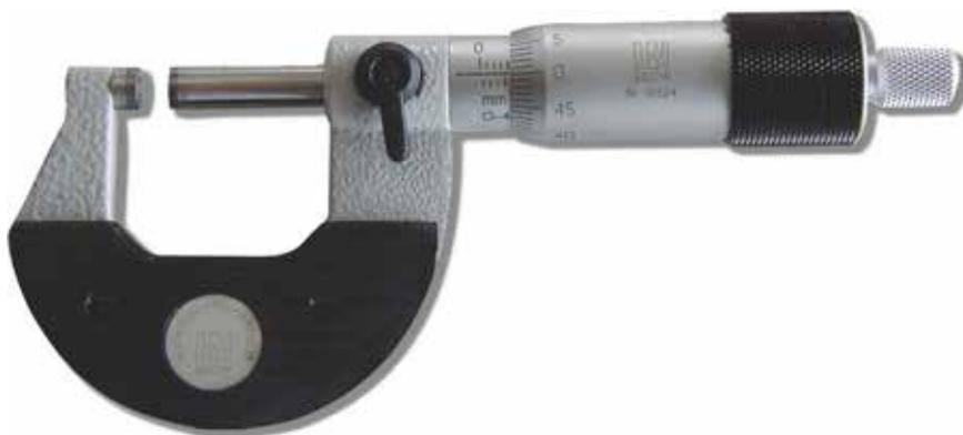
**High quality/accuracy outside micrometer.** Casting painted arc heat-insulated. Thimble (Ø 18 mm) chromed and etched by laser for a clear and long lasting. Friction on the thimble and locking lever. Screw completely hardened and ground with specific working systems to assure the max accuracy for a long time. Serial number. Manufactured as per DIN 863. Supplied in a box with key and setting rod. Carbide contacts.
