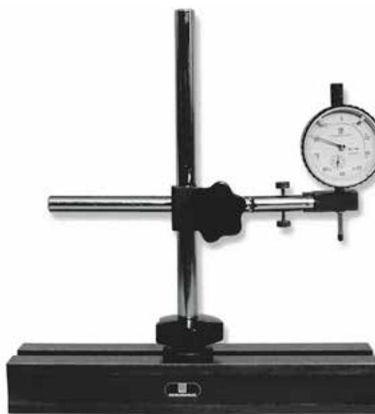
**Dial indicator stand with prismatic base in cast iron entirely ground on the resting points.** T-slot for moveable dial indicator holder rod. V-groove for resting on rounded surfaces. Dial indicator connector with fine adjustment screw. Columns in chromed steel. Supplied without dial indicator.
