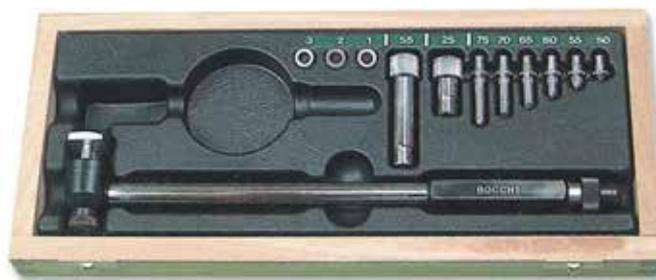
**High precision bore gauges** suitable for measuring ovality and taper of bores. Good transmission of movement. Contact points in hardened steel. Body in chromed steel with heat-insulated grip. Manufactured as per DIN 878. Supplied in case without dial indicator. Available upon requirement: **Art. 5271 version with carbide contact points.**
