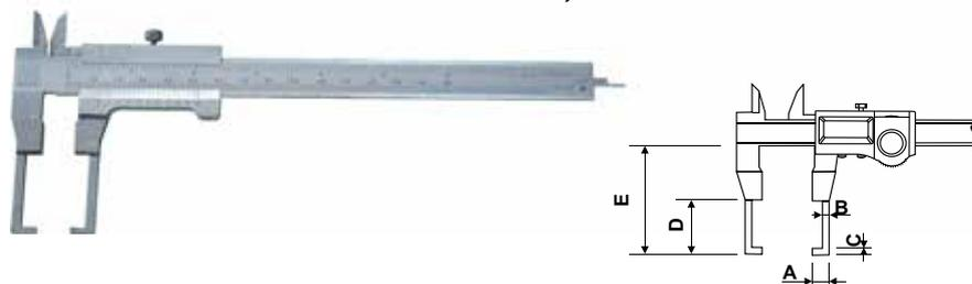
**Digital caliper** in hardened stainless steel. 5 figure liquid crystal display and minus sign. mm/inch conversion. Set to zero in any position. RS232C output to printer port. Slider locking screw. Battery powered. Automatic switch-off. **Suitable for measuring grooves and external seatings.** Serial number. Manufactured as per DIN 862. Supplied in case.
