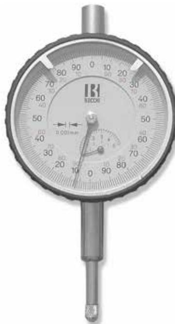
*Entirely shockproof, high precision dial indicator with measurement to 0,001 mm. Ruby-mounted gear movements for absolute precision. Rotating bezel with tolerance markers. Manufactured as per DIN 879.*
