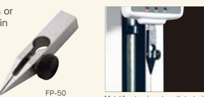
Metal line tension strength test with FP-51.
