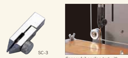
Copper foil peeling test with SC-8.
