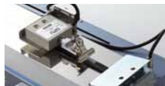
Peel test of embossed carrier tape
