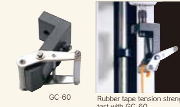
Rubber tape tension strength test with GC-60.
