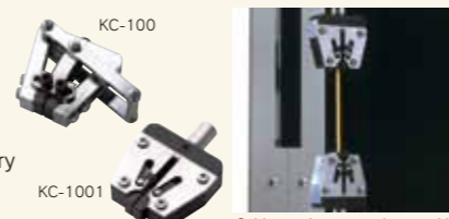
Cable tension strength test with KC-1001.
