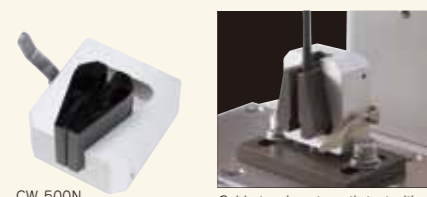
Cable tension strength test with CW-500N.
