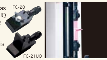
180 degree peel testing of adhesive tapes with FC-21
