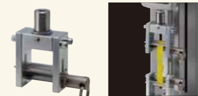
PP band tension strength test with PPC-5000N.
