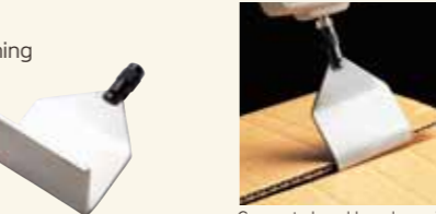
Corrugated card board opening strength test with DF-60
